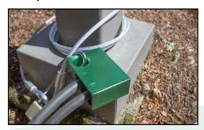
Field set-up is a breeze in all weather and space conditions. Set road tubes for counting one or two lanes, attach them to the Road Runner, and lock it on the roadside. The unit is always counting.
